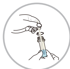
Insert the swab with specimen into the dilution buffer and stir swab at least 10 times
